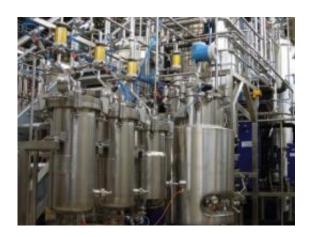
The new fermentation plant transforms the processes of producing enzymes to industrial scale. Credit: © Fraunhofer
