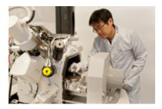
The tiny patterns are formed on the gold surface using a process called ion beam milling (the focused ion beam system is used to create nanoscale intaglio metamaterial patterns on the metal surface.
