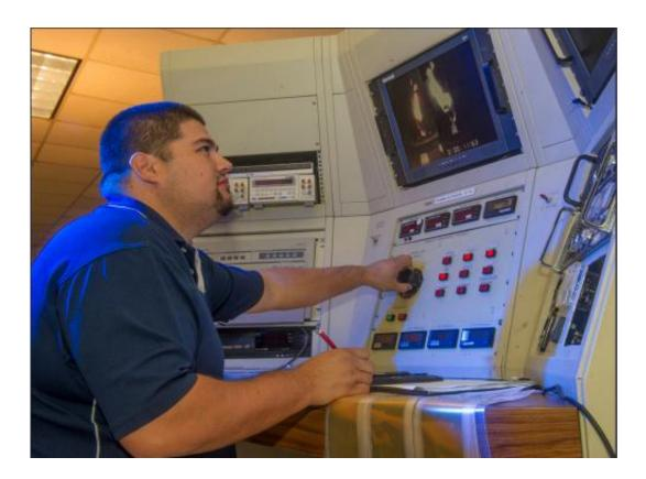
Erick Ordonez, a structural materials engineer at the Marshall Center, controls the levels of nitrogen and oxygen going into the chamber during a fire demonstration test. Credit: NASA/MSFC/Emmett Given
