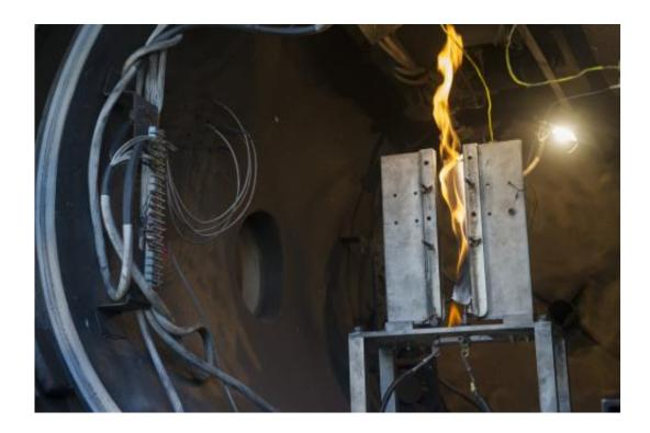
During a combustion demonstration test, a sample material is set on fire for 30 seconds in a large chamber, filled with varying pressure levels of nitrogen and oxygen. Data, including the maximum oxygen concentration at which a propagating flame will go out, is collected while the samples are kindled for 30 seconds. The test data will be important in the design of a future, large-scale fire experiment in space. Credit: NASA/MSFC/Emmett Given
