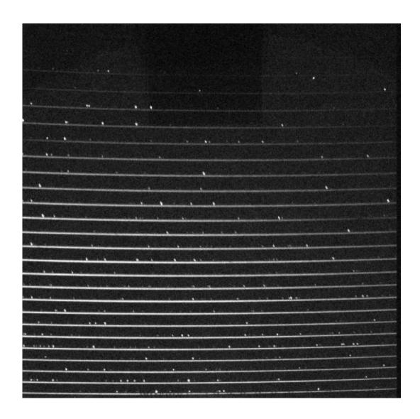
This is a first light image of Vega from LCOGT's prototype NRES. The continuous lines across the image is the spectra of the star. The spots are from the Thorium Argon calibration light. Credit: LCOGT
