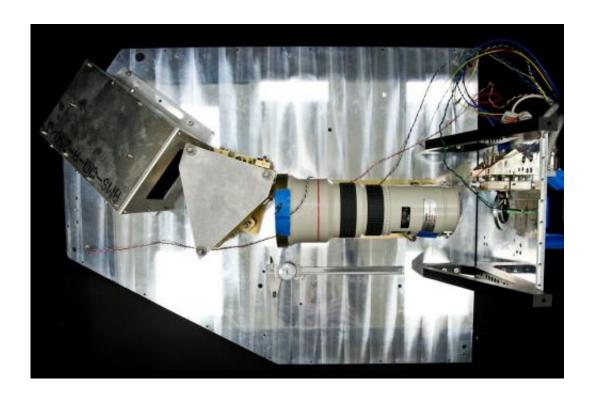
This is a NRES prototype out of its housing in the LCOGT lab. Credit: Jason Eastman
