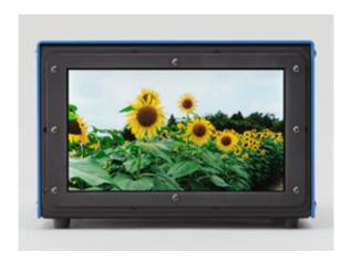
(Phys.org)—Japanese firm Ortus Technology Co., Ltd. has revealed its development of what the company is calling the world's smallest LCD display panel that meets the 4K standard. At just 9.6 inches with a resolution of 3,840 x 2,160 pixels, the new display will be small enough for use in handheld devices.
