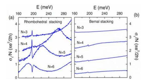
The infrared absorption due to both electronic transitions and phonons in fewlayer (3 to 6 layers) graphene samples having rhombohedral (left) and Bernal (right) layer stacking. The highly asymmetric phonon contribution near 200 meV is a result of the coupling between the electrons and phonons.
