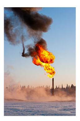
Flares burn off excess methane at oil and gas refineries, landfills, and other industrial plants. Flares are used to control release of methane into the atmosphere but recovery options are also available that capture methane for use as fuel.
