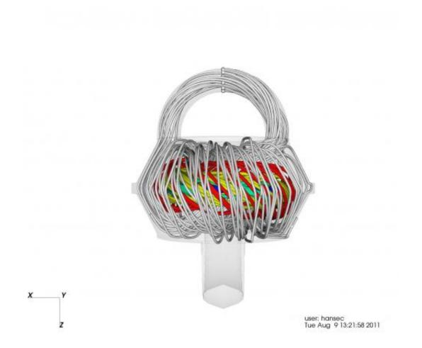
Alternating the current through the handles produce asymmetric magnetic fields, shown here, which act to contain the plasma. Credit: T. Jarboe, Univ. of Washington
