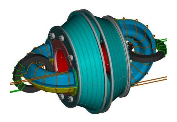
This is a computer drawing of the prototype, which attaches current-carrying handles to either end of the central plasma. Credit: T. Jarboe, Univ. of Washington
