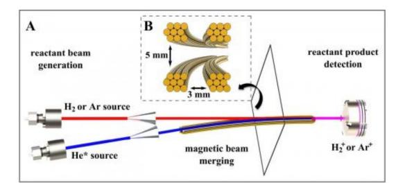
The experimental system is comprised of two supersonic valves followed by two skimmers. The blue beam passes through a curved magnetic quadrupole guide, and the merged beam (purple) enters a quadrupole mass spectrometer. B is a front view of the quadrupole guide. Credit: Weizmann Institute of Science
