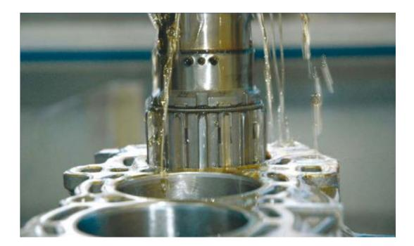
The honing tool adjusts its shape to match the piston bore holes. Credit: Fraunhofer IWU
