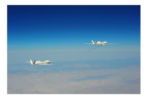
Currently global military aviation relies on a key enabler – aerial refueling. Fighters, bombers, reconnaissance and transport aircraft use "flying gas stations" to go the extra mile. Increasingly, UAVs are conducting combat and ISR operations, but UAVs aren't designed to be refueled in flight. In 2007, DARPA teamed up with NASA to show that high-performance aircraft can easily perform automated refueling from
