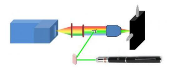
This is a schematic drawing of the Raman spectrometer, including a laser pointer, dichroic mirror, prism, objective, x,y motorized translational stage, long wavepass edge filter, lens and a detector (spectrometer/intensified charge-coupled device). Credit: Ilana Bar, Ben Gurion University of the Negev
