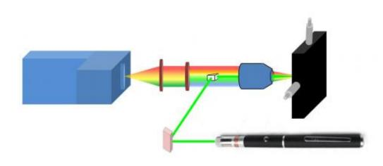
This is a schematic drawing of the Raman spectrometer, including a laser pointer, dichroic mirror, prism, objective, x,y motorized translational stage, long wavepass edge filter, lens and a detector (spectrometer/intensified chargecoupled device). Credit: Ilana Bar, Ben Gurion University of the Negev
