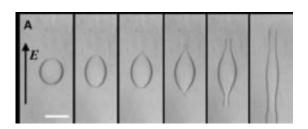
This shows the deformation of a droplet as the voltage increases. Credit: Xuanhe Zhao
