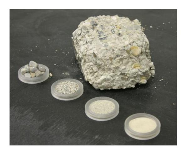
Researchers have developed a method of breaking down concrete into its constituent parts. Credit: Fraunhofer IBP
