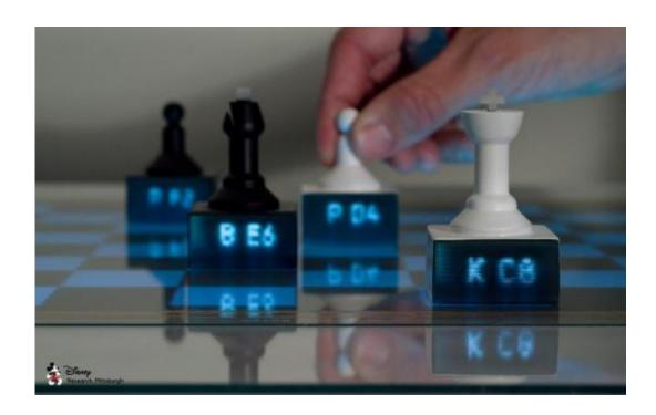
Chess pieces with embedded light pipes display content piped from an interactive tabletop. Contextual information, such as chess piece location and suggested moves, can be displayed on each individual piece.
