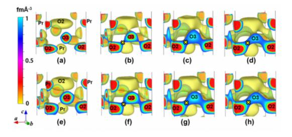
Temperature dependence of the isosurface of nuclear density in (a–d)  $Pr_2Ni_{0.75}Cu_{0.25}O_{4+\delta}$  and (e–h)  $Pr_2(Ni_{0.75}Cu_{0.25})_{0.95}Ga_{0.05}O_{4+\delta}$ . O2 and O3 stand for the apical and interstitial oxygen atoms, respectively. × denotes the bottleneck with the minimum nuclear density on the O2-O3 diffusion path. (a) 25 °C, (b) 602 °C, (c) 807 °C, (d) 1011 °C, (e) 20 °C, (f) 605 °C, (g) 810 °C, (h) 1011 °C.
