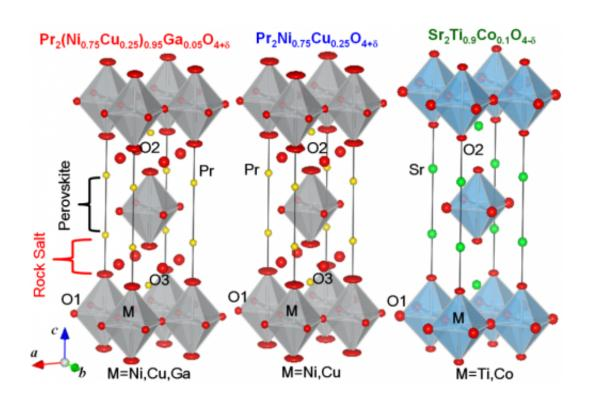
Refined crystal structures of  $Pr_2(Ni_{0.75}Cu_{0.25})_{0.95}Ga_{0.05}O_{4+\delta}$ ,  $Pr_2Ni_{0.75}Cu_{0.25}O_{4+\delta}$ , and  $Sr_2Ti_{0.9}Co_{0.1}O_{4-\delta}$ , which were obtained by the Rietveld analysis of neutron-diffraction data taken at room temperature.  $Pr_2(Ni_{0.75}Cu_{0.25})_{0.95}Ga_{0.05}O_{4+\delta}$  and  $Pr_2Ni_{0.75}Cu_{0.25}O_{4+\delta}$  have the excess interstitial O3 atoms.
