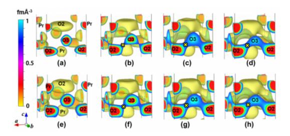
Temperature dependence of the isosurface of nuclear density in (a–d)  $Pr_2Ni_{0.75}Cu_{0.25}O_{4+\delta} \text{ and (e-h)} \ Pr_2(Ni_{0.75}Cu_{0.25})_{0.95}Ga_{0.05}O_{4+\delta}. \ O2 \ and \ O3 \ stand for the apical and interstitial oxygen atoms, respectively. × denotes the bottleneck with the minimum nuclear density on the O2-O3 diffusion path. (a) 25 °C , (b) 602 °C, (c) 807 °C, (d) 1011 °C, (e) 20 °C, (f) 605 °C, (g) 810 °C, (h) 1011 °C.$
