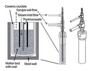
Molten catalytic reactor design. Steam and coal react in a bed of molten alkali salts. Isometric and cutaway views. (Furnace not shown.)
