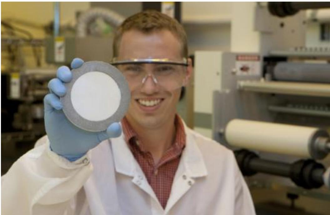
Matthew Hagedon with electrofluidic imaging film. The white, plastic film, ten times thinner than a sheet of paper, is in a rigid frame for support during lamination into a display. The goal is a large roll of film that can be laminated onto electronics. Credit: Lisa Ventre
