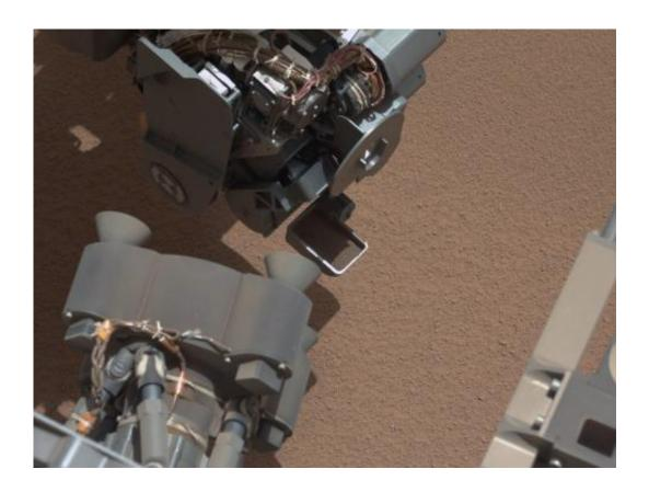
This image from the right Mast Camera (Mastcam) of NASA's Mars rover Curiosity shows a scoop full of sand and dust lifted by the rover's first use of the scoop on its robotic arm. In the foreground, near the bottom of the image, a bright object is visible on the ground. The object might be a piece of rover hardware. This image was taken during the mission's 61st Martian day, or sol (Oct. 7, 2012), the same sol as the first scooping. After examining Sol 61
