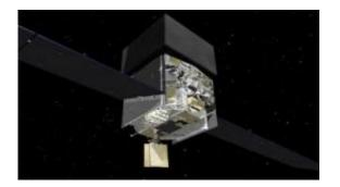
This computer graphic shows the structure of NASA? Fermi satellite. The central, box-shaped instrumentation platform lies between the solar panels. The Large Area Telescope, whose data the astronomers evaluated, is hidden beneath the black cover visible on the top. Credit: NASA
