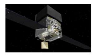
This computer graphic shows the structure of NASA?s Fermi satellite. The central, box-shaped instrumentation platform lies between the solar panels. The Large Area Telescope, whose data the astronomers evaluated, is hidden beneath the black cover visible on the top. Credit: NASA
