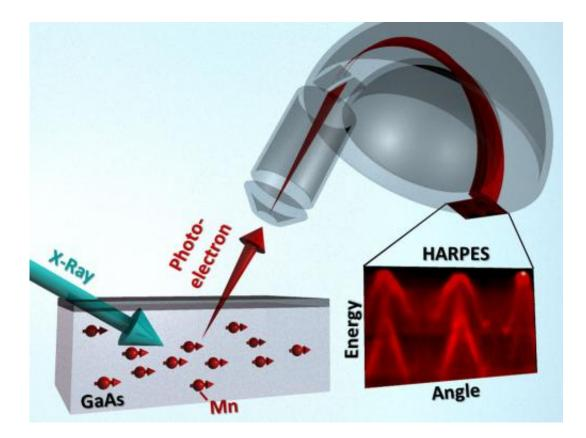
With the HARPES technique, a beam of hard x-rays flashed on a sample causes photoelectrons from within the bulk to be emitted. Measuring the kinetic energy of these photoelectrons and the angles at which they are ejected reveals much about the sample? selectronic structure. Here the Mn atoms in GaMnAs are shown to be aligned ferromagnetically, with all their atomic magnets pointing the same way. Credit: Alex Gray, Stanford and SLAC
