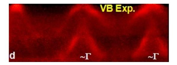
HARPES data on GaMnAs indicate that the ferromagnetism of dilute magnetic semiconductors arise from two distinct mechanisms.
