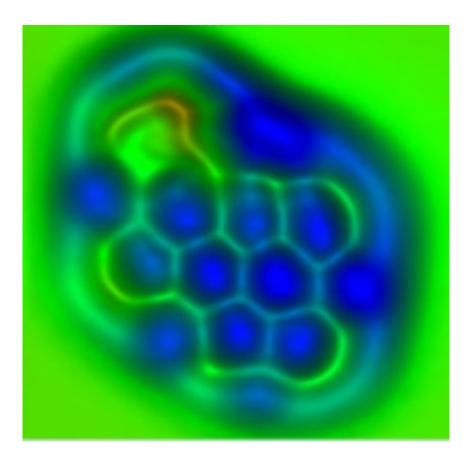
This is a nanographene molecule exhibiting carbon-carbon bonds of different length and bond order imaged by noncontact atomic force microscopy using a carbon monoxide functionalized tip. This molecule was synthesized by Centro de Investigación en Química Biolóxica e Materiais Moleculares (CIQUS) at the Universidade de Santiago de Compostela. Credit: IBM
