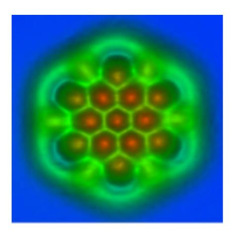
A nanographene molecule exhibiting carbon-carbon bonds of different length and bond order imaged by noncontact atomic force microscopy using a carbon monoxide functionalized tip. This molecule was synthesized at the Centre National de la Recherche Scientifique (CNRS) in Toulouse. Credit: IBM
