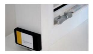
The sensor nodes embedded in the window frame transmit the data via the s-net wireless sensor. The prototype of the RF node (left) pictured here will be installed in the sensor housing (right) of the finished system. Credit: © Fraunhofer IIS
