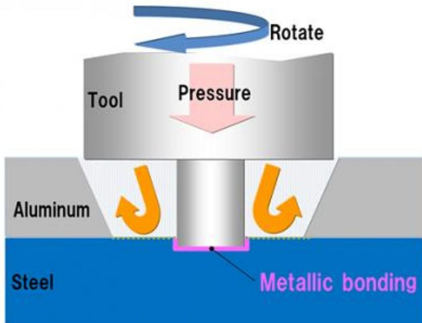
Conceptual diagram of FSW of dissimilar metals.
