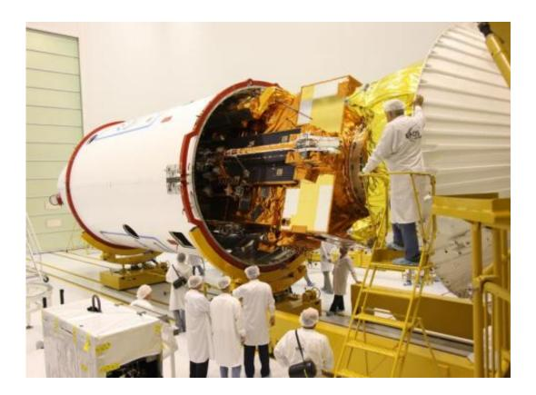
Last view of MetOp-B as it is eased into the rocket fairing for launch on 17 September 2012. Credits: ESA
