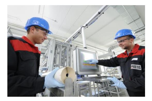
The membrane elements for water treatment are manufactured in the semiautomatic system in Bitterfeld. A single membrane element consists of a bundle of over 20 layers. It is aligned with a winding module and secured. The LANXESS employee (left) is holding such a module. Credit: LANXESS AG
