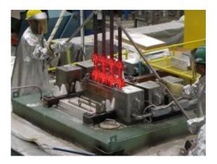
Argonne researchers Osman Eryilmaz (left) and Vivekanand Sista (right) recover industrial parts from the large-scale ultra-fast boriding furnace after a successful boriding treatment. The furnace uses an electrochemical process similar to that of batteries to deposit boron on metal workpieces. Photo credit: Osman Eryilmaz
