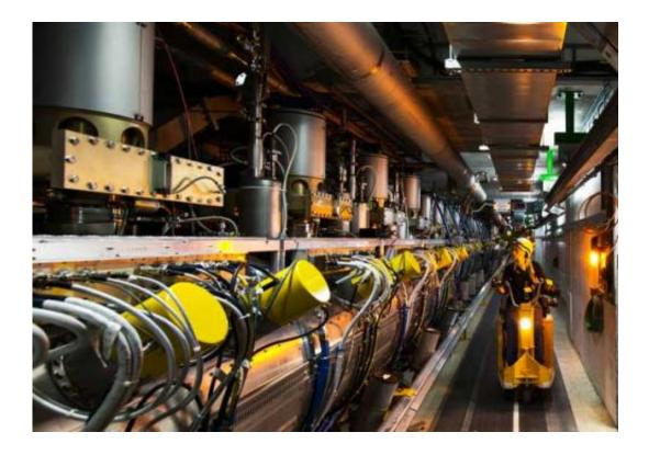
Radiofrequency cavities in the LHC tunnel had be retuned to accelerate protons and lead ions. Credit: CERN
