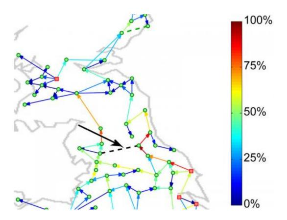
A line in the wrong place: If the British grid operators were to lay a new power line along the broken line (arrow), they would apparently be closing a gap in the grid. Based on Braess's Paradox, however, this new line would disrupt power transmission throughout the network. Credit: Dirk Witthaut and Marc Timme / MPI for Dynamics and Self-Organisation
