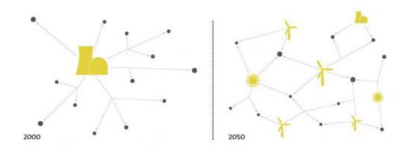
The energy transformation as a supply grid issue: Currently, large central power plants basically supply their immediate surroundings. In future, more small, decentralized wind and solar generators will take on a greater load of the supply. This will lead to a new network architecture that may be less vulnerable to power outages than present-day grids, contrary to the fears of some. Credit: designergold, based on outlines provided by the MPI for Dynamics and Self-Organization
