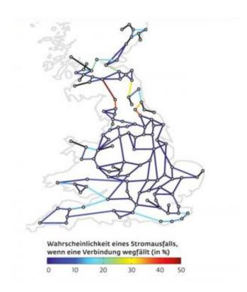
How robust is the power grid? Using the British grid as an example, the Göttingen-based scientists calculated what happens when individual lines are cut. If one of the blue lines is cut, an outage in the whole network is unlikely. In the case of the dark red lines, however, the likelihood of a total blackout rises to almost 50 per cent. Credit: Dirk Witthaut and Marc Timme / MPI for Dynamics and Self-Organisation
