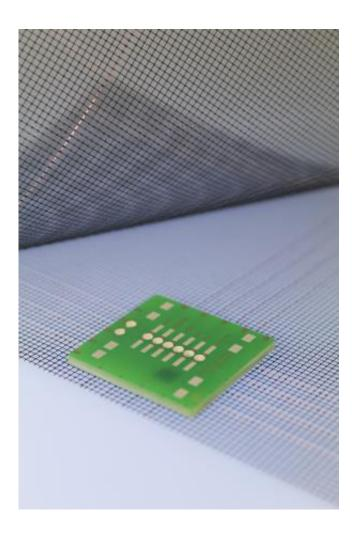
A smart fabric incorporating conductive threads and a processor module provides protection against intrusion and theft.
