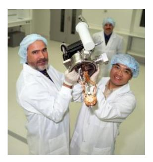
Team leader David Jamieson (left) with Changyi Yang in the CQC2T cleanrooms at the University of Melbourne with the special quantum computer device chip holder ready to be loaded into the ion implantation system. Credit: University of Melbourne
