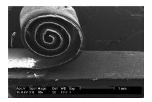
The silicon/copper/polymer composite can be rolled from its silicon substrate and leave a mask in place to begin anew the process of making another anode for a lithium-ion battery. Credit: Alexandru Vlad/Rice University
