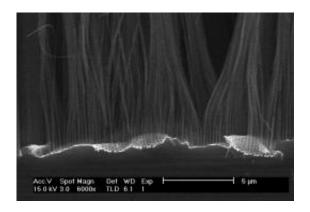
As silicon is dissolved in a chemical bath, a gold mask sinks to the bottom, leaving silicon nanowires about 100 nanometers wide poking through the holes. Because silicon holds as much as 10 times the lithium as the anode in a typical lithium-ion battery, researchers at Rice University and in Belgium are researching ways to recycle waste silicon into functional battery components. Credit: Alexandru Vlad/Rice University
