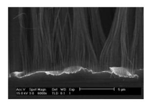
As silicon is dissolved in a chemical bath, a gold mask sinks to the bottom, leaving silicon nanowires about 100 nanometers wide poking through the holes. Because silicon holds as much as 10 times the lithium as the anode in a typical lithium-ion battery, researchers at Rice University and in Belgium are researching ways to recycle waste silicon into functional battery components. Credit: Alexandru Vlad/Rice University
