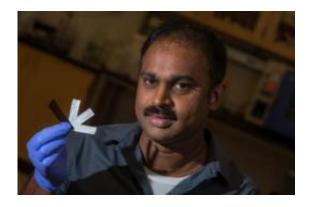
Rice University research scientist Arava Leela Mohana Reddy holds strips of anode material and a piece of waste silicon (at left). Researchers at Rice and in Belgium found a way to recycle silicon into flexible anodes for lithium-ion batteries. Credit: Jeff Fitlow, Rice University
