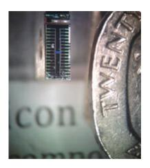
Example of a silicon quantum chip next to a 20 pence coin.
