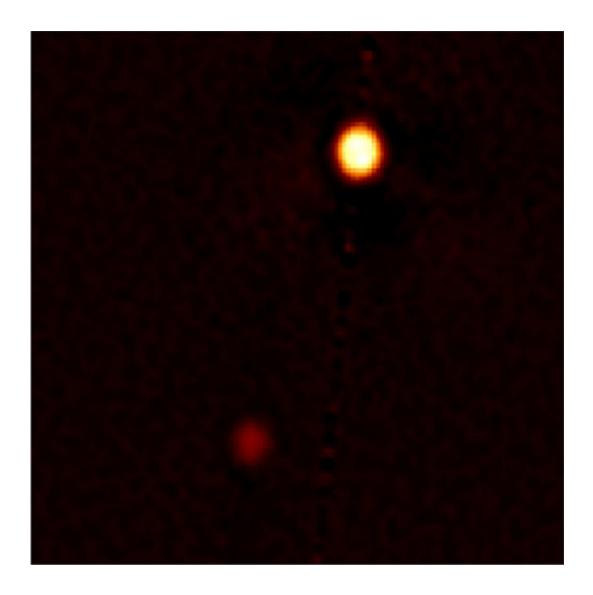
Speckle image reconstruction of Pluto and Charon obtained in visible light at 692 nanometers (red) with the Gemini North 8-meter telescope using the Differential Speckle Survey Instrument (DSSI). Resolution of the image is about 20 milliarcseconds rms (root mean square). This is the first speckle
