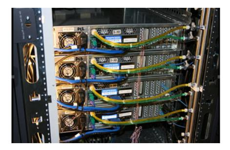
Closeup of the back of the server rack with Cool-Flo installed. The coolant flows through the tubes into the server and carries the heat out like a circulatory system.
