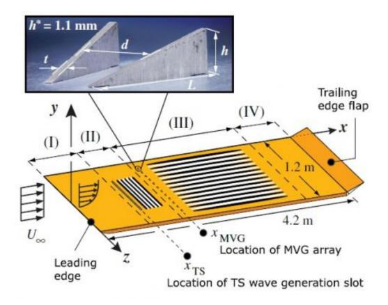
Illustration of the flat plate used in tests, with a photo by John Hallmen of a pair of miniature vortex generators. Image credit: Shahinfar, et al. ©2012 American Physical Society
