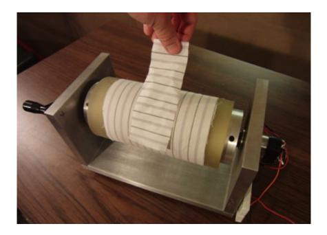
To create a model of friction sounds, researchers hold a piece of cloth against a motorized cloth roller. Ultimately, rotor speed will be matched to the speed of movement in an animation.
