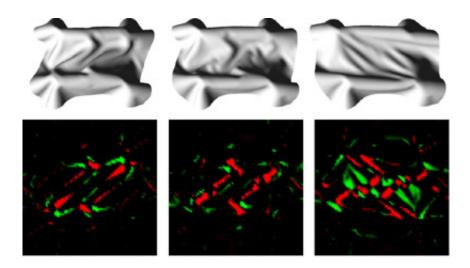
To match sound to action, a computer looks at frames of computer animation of a piece of fabric and measures how much parts of the image are raised or lowered as a basis for synthesizing "crumpling" sound.
