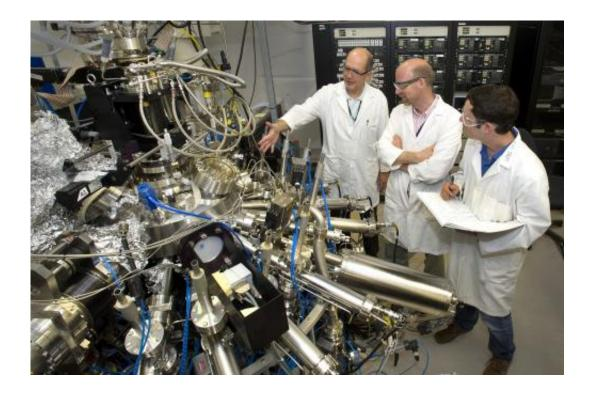
Physicist Ivan Bozovic (left) describes the real-time feedback of his custom-built molecular-beam epitaxy (MBE) machine, which built the near-flawless samples critical to this experiment, to collaborating physicists John Hill (center) and Mark Dean (right).
