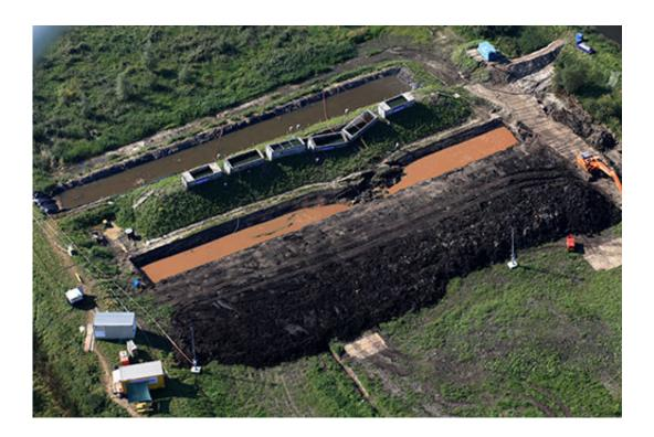
(Phys.org)—Civil engineers from Rensselaer Polytechnic Institute were part of an international research team that collapsed a full-scale dike this week in The Netherlands. The test dike was embedded with advanced sensors and traditional measurement instruments, and results of the study are expected to help validate powerful new technologies for monitoring the health of aging flood-control infrastructure.
