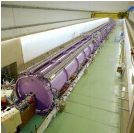
Cosmic radiation is produced with the GSI linear accelerator. Credit: A. Zschau / GSI Helmholtzzentrum für Schwerionenforschung
