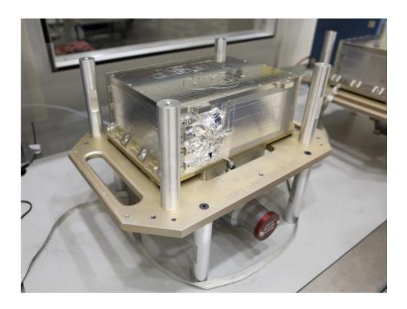
The Relativistic Electron Proton Telescope (REPT) instrument of the Energetic Particle, Composition, and Thermal Plasma Suite (ECT) for RBSP spacecraft B, shown prior to installation. Credit: JHU/APL
