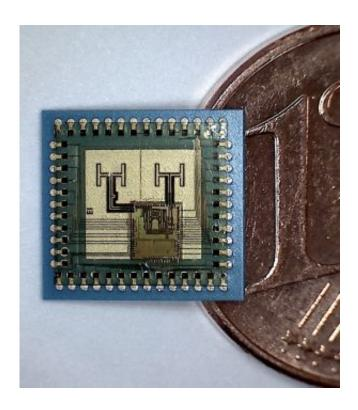
The novel radar sensor has only half the size of a Euro cent coin but contains all necessary radio-frequency components. Credit: Robert Bosch GmbH/SUCCESS
