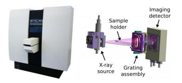
Together with industry partner Bruker microCT / Skyscan, a team of university researchers led by scientists at the Technische Universitaet Muenchen has developed a preclinical x-ray scanner (left) with enhanced contrast for soft tissue imaging. Mounted in a movable gantry inside the scanner are (right) an x-ray source, a detector, and a three-grating interferometer for phase-contrast imaging. Copyright Arne Tapfer, TU Muenchen
