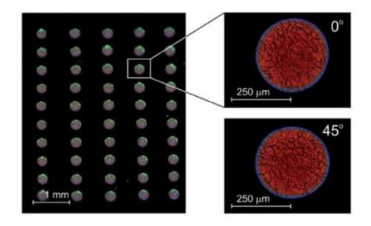
Pictures of inkjet-printed LC laser droplets on a PVA film.
