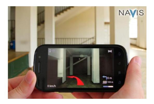
NAVVIS uses realistic 3D images to point users in the right direction. Credit: G. Schroth/TUM
