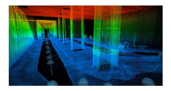
For the mapping NAVVIS uses both vertical and horizontal laser scans. The environment is displayed as a three-dimensional point cloud. Credit: G. Schroth/TUM
