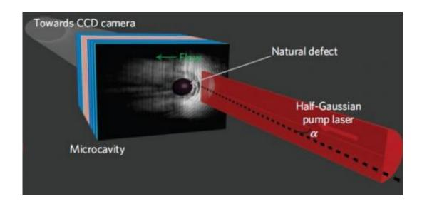
Experimental set-up showing the injection of a polariton fluid and the formation of half-solitons, which act like magnetic monopoles. Image credit: R. Hivet, et al. ©2012 Macmillan Publishers Limited
