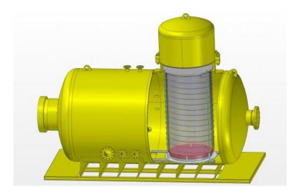
This is a drawing of the container used to study convection. The 8-foot tall cylinder was heated at the bottom and cooled at the top. Credit: UCSB
