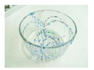
A reconstructed fractured soda lime silicate Pyrex bowl. Arrows outline crack paths. Credit: George Quinn
