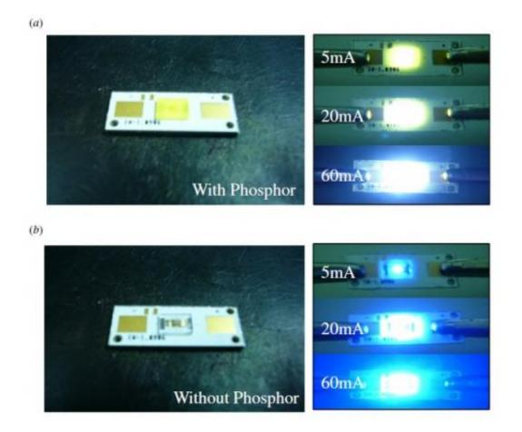
Tests demonstrate the improved performance for the LED chips packaged inside a glass substrate with phosphor molding (a) compared to those without phosphor molding (b). Credit: Chang-Chien, et al. ©2012 IOP Publishing Ltd
