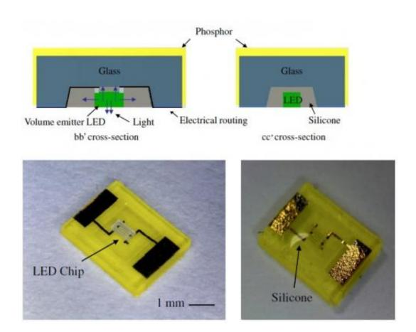
(Top) Two cross-sectional views of an LED packaged inside a transparent glass substrate with a phosphor coating. (Bottom) Images of the LED package before (left) and after (right) silicone is added. Credit: Chang-Chien, et al. ©2012 IOP Publishing Ltd
