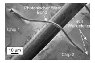
The wire bond is adapted to the position and orientation of the chips. Credit: Figure: N. Lindenmann and G. Balthasar
